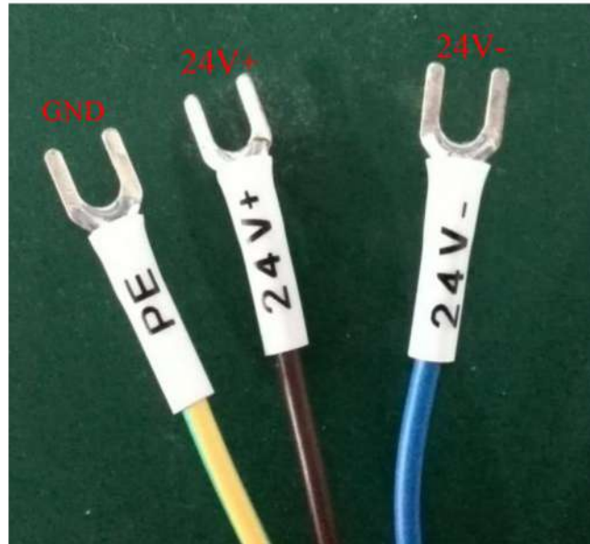
Figure 3. Definition of power line wires
